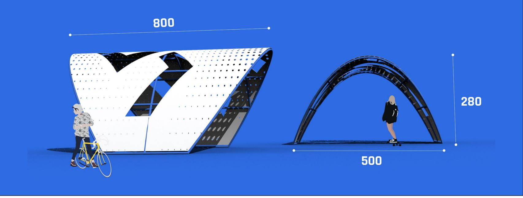
The objective was to design and construct two pavilions for the Kuwait Marathon 2019. The pavilions were inspired by Kuwait Marathon logo. The pavilions were constructed from a curved steel frame with perforated aluminum panels.
